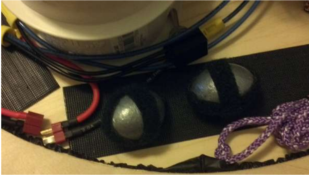
Figure 2 - 8oz lead fishing weights used to balance SARAH.
